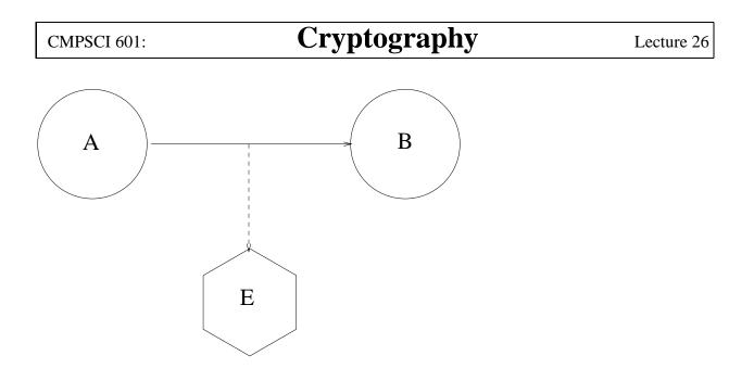
**One-Time Pad:**  $p \in \{0,1\}^n$ ;  $m \in \{0,1\}^n$   $E(p,x) = p \oplus x$   $D(p,x) = p \oplus x$  $D(p,E(p,m)) = p \oplus (p \oplus m) = m$
