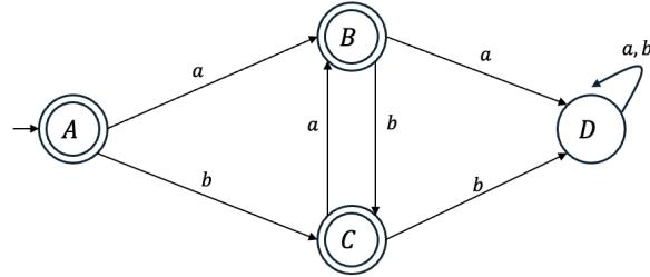
State set  $\{A, B, C, D\}$ , start state  $A$ , final state set  $\{A, B, C\}$ , transitions  $\delta(A, a) = B$ ,  $\delta(A, b) = C$ ,  $\delta(B, a) = D$ ,  $\delta(B, b) = C$ ,  $\delta(C, a) = B$ ,  $\delta(C, b) = D$ ,  $\delta(D, a) = \delta(D, b) = D$ .
