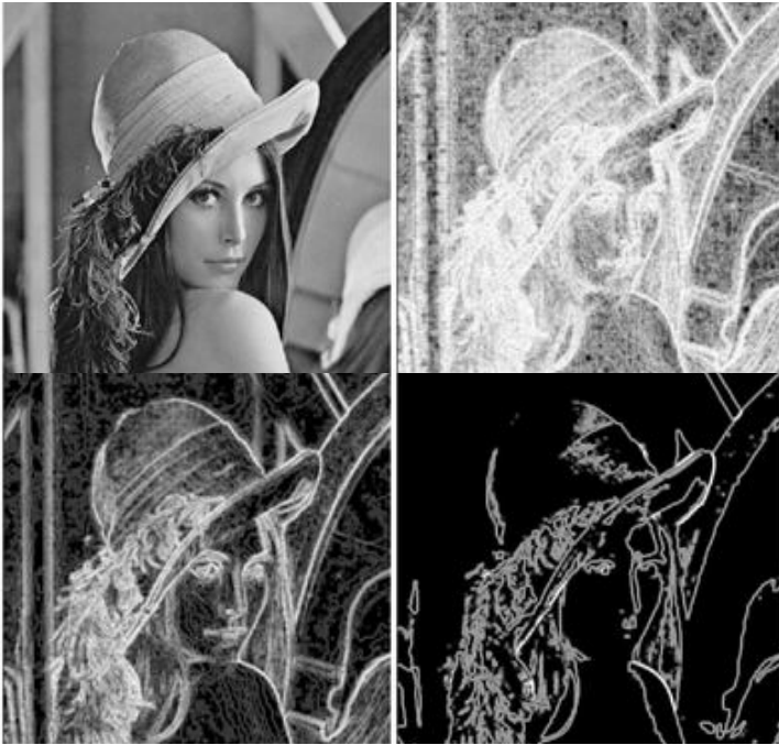
Fig. 2. Sketching the defined complexity function for different number of quantizing levels: (a) top-left: original image, (b) top-right: no quantization, (c) bottom-left: 32 levels of quantization and (d) bottom-right: 2 levels of quantization.
