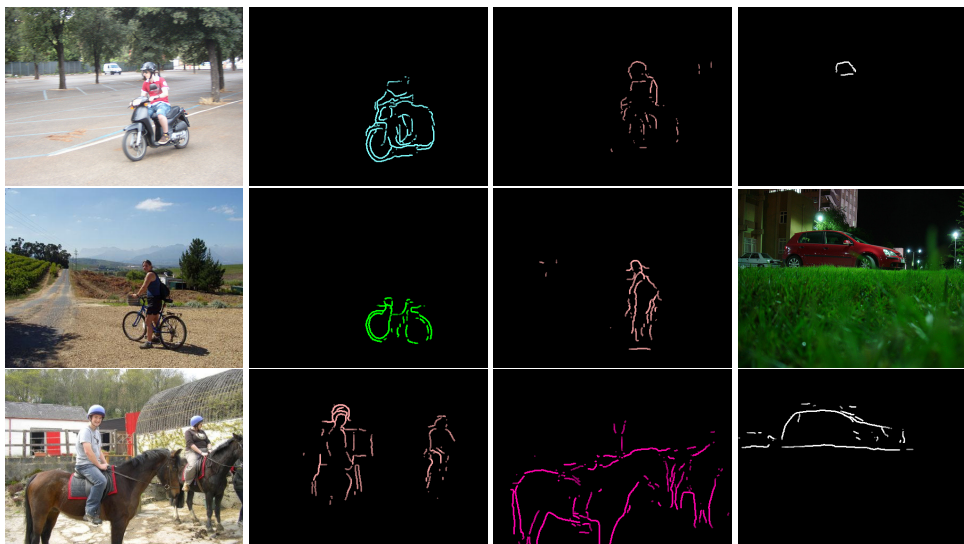
Figure 7. Results on semantic contour detection. The category is indicated by the color(motorbike: blue, car: gray, bicycle: green, horse: magenta, person: pink), following the PASCAL convention.
