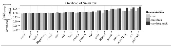
Figure 6. Overhead of STABILIZER relative to runs with randomized link order (lower is better). With all randomizations enabled, STABILIZER adds a median overhead of 6.7%, and below 40% for all benchmarks.
