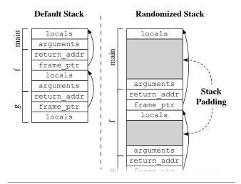
**Figure 4.** STABILIZER randomizes the stack by adding up to a page of random padding at each function call. Functions are instrumented to load a pad size from the stack pad table. STABILIZER periodically refills this table with new random values to re-randomize the stack.
