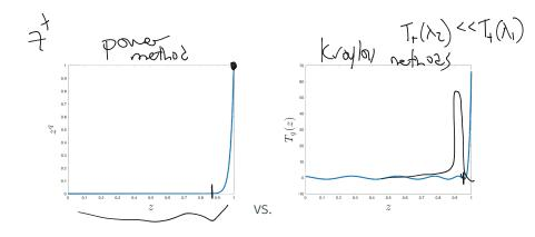
Optimal 'jump' polynomial in general is given by a degree *t* Chebyshev polynomial. Krylov methods find a polynomial tuned to the input matrix that does at least as well.
