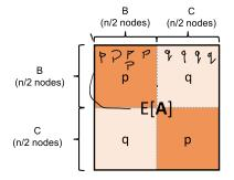
$G_n(p,q)$ : stochastic block model distribution. B,C: groups with n/2 nodes each. Connections are independent with probability p between nodes in the same group, and probability q between nodes not in the same group.
