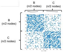
$G_n(p,q)$ : stochastic block model distribution. B,C: groups with n/2 nodes each. Connections are independent with probability p between nodes in the same group, and probability q between nodes not in the same group.
