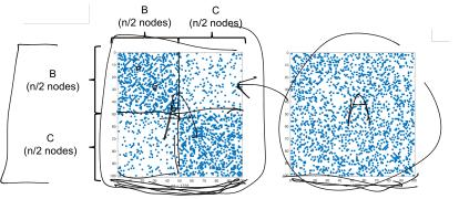
$G_n(p,q)$ : stochastic block model distribution. B,C: groups with n/2 nodes each. Connections are independent with probability p between nodes in the same group, and probability q between nodes not in the same group.
