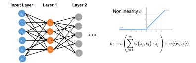
• Evaluating  $\mathcal{N}(x)$  requires  $|x| \cdot |\text{layer 1}| + |\text{layer 1}| \cdot |\text{layer 2}| + \dots$  multiplications if fully connected.
