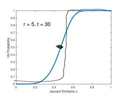
r and t are tuned depending on application. 'Threshold' when hit probability is 1/2 is  $\approx (1/t)^{1/r}$ . E.g.,  $\approx (1/30)^{1/5} = .51$  in this case.
