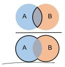
Natural measure for similarity between bit strings – interpret an n bit string as a set, containing the elements corresponding the positions of its ones.  $J(x, y) = \frac{\# \text{ shared ones}}{\text{total ones}}$ .
