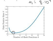
False Positive Rate: with m bits of storage, k hash functions, and n items inserted  $\delta \approx \left(1 - e^{\frac{-kn}{m}}\right)^k$ .
