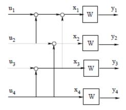
After m steps of the above recursion we obtain a collection of  $2^m$  channels. We randomly pick one of these channels and denote its capacity by  $I_m$ . In this part we establish convergence properties of the random process  $I_m$ . The sequence of random variables  $I_m$  converges almost surely to a Bernoulli 0-1-valued random variable  $I_\infty$  such that:
