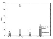
Fig. 12: Execution time for the WAN-Experiment benchmark on 50 cluster nodes plus a remote server.
