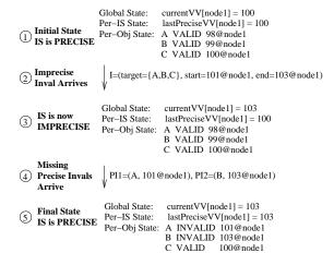
Fig. 5: Example of maintaining interest set state. For clarity, we only show node1's elements of *currentVV* and *lastPreciseVV*.
