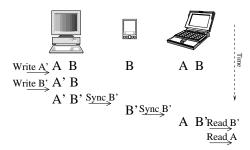
Fig. 2: Naive addition of PR to an AC-TI log exchange protocol fails to provide consistency.
