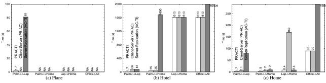
Fig. 10: Synchronization time among devices for different network topologies and protocols.
