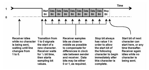
The receiver samples as close to the middle of a bit as possible to avoid measuring the line as a bit is changing from 0 to 1 or from 1 to 0. This also compensates for slight differences in clock rates between sender and receiver. For 8-bit characters a difference of a few percent can be tolerated without dropping data.
