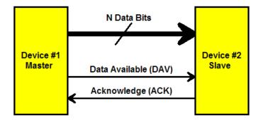
The process of communicating data from one device to another using this approach is called *handshaking*. The master places new information onto the data lines, and then *raises* the DAV data available line, making it go from 0 to 1. When the slave sees DAV go high, it acknowledges by raising the ACK line and latching the data into its receive buffer. When the master sees ACK go high, it lowers DAV go low, it lowers ACK. As soon as the master sees ACK go low it knows that the cycle is complete.
