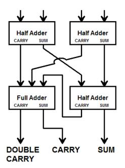
By extending this process even further, we will find that the adders for the partial product columns get more and more complicated. We can extend the quad adder to a "quint adder" by replacing one of the input half adders with a full adder, and then extend it again to a "hex adder" by replacing both of them, as shown below:
