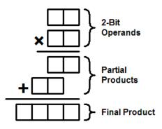
In binary each partial product is generated by multiplying an operand by either 0 or 1, resulting in either zero or a copy of the operand. This is the same behavior as a group of AND-gates. One 2-input AND-gate is used for each pair of bits, then the bits are added together with half-adders and full-adders to generate the final product. The hardware for multiplying two 2-bit numbers together is shown below:
