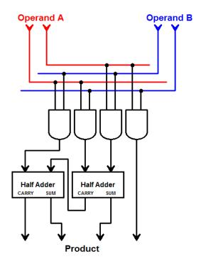
To add the partial products the circuit requires only a pair of half-adders, the leftmost accepting a carry out of the rightmost. Notice that the rightmost partial product bit appears in the answer directly; this will be the case for the product of two numbers of any length.
