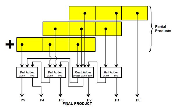
Notice that the quad adder circuit returns a 3-bit sum, emitting the sum bit to the answer, a carry bit to the next stage of partial products, and a *double-carry* to the stage beyond that.
