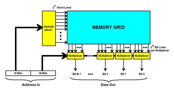
For example, a 64K byte memory system requires 16 address bits and 8 data bits. The grid contains  $2^{16} \times 2^3 = 2^{19}$  data bits. Arranging the memory as 64K rows (word lines) by 8 columns (bit lines) requires a demultiplexer with  $2^{16}$  AND-gates, each with 16 inputs, and no multiplexers. This is 65536 separate AND-gates.
