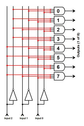
The example shown has three inputs, so it must have  $2^3$ =8 outputs, numbered from 0 to 7. Every binary pattern activates exactly one of the AND-gates. Every AND-gate in the example is inscribed with the number that corresponds to its binary trigger value. Place any binary value on the input lines and trace the signal flow through the circuit to prove to yourself that only a single AND-gate is ever activated.
