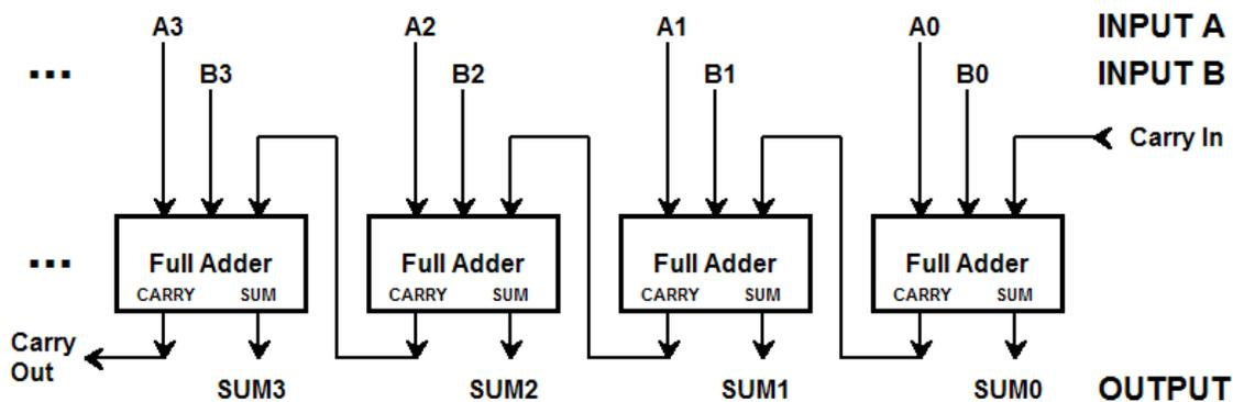
Normally for addition the Carry In bit is 0. For us to use the adder as a subtractor we need only form the two’s complement of input B. This can be done by complementing all the input bits of B (forming the one’s complement), and setting the Carry In bit to 1.
