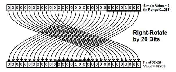
The trick to forming constants in this manner is to first insure that the desired constant has all of its 1-bits constrained to an 8-bit block, shown by the thick line in the diagram. If the 1-bits fit into an 8-bit block *and* the count of 0-bits to the right of the block is an even number, then the constant can be formed.
