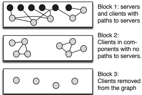
Figure 1: Separating a Client-Server Graph into blocks
