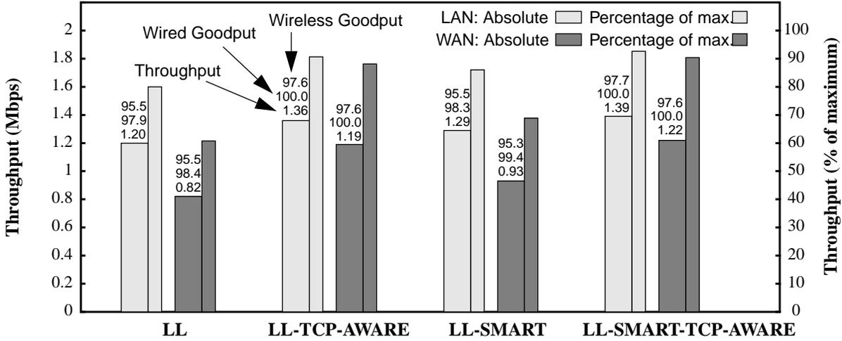
Figure 11. Performance of link-layer protocols: bit-error rate =  $1.9 \times 10^{-6}$  (1 error/65536 bytes), socket buffer size = 32 KB. For each case there are two bars: the thick one corresponds to the scale on the left and denotes the throughput in Mbps; the thin one corresponds to the scale on the right and shows the throughput as a percentage of the maximum, i.e. in the absence of wireless errors (1.5 Mbps in the LAN environment and 1.35 Mbps in the WAN environment).
