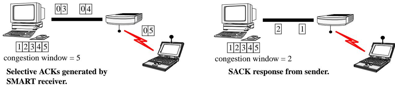
**Figure 3. TCP with SMART-based selective acknowledgements**
