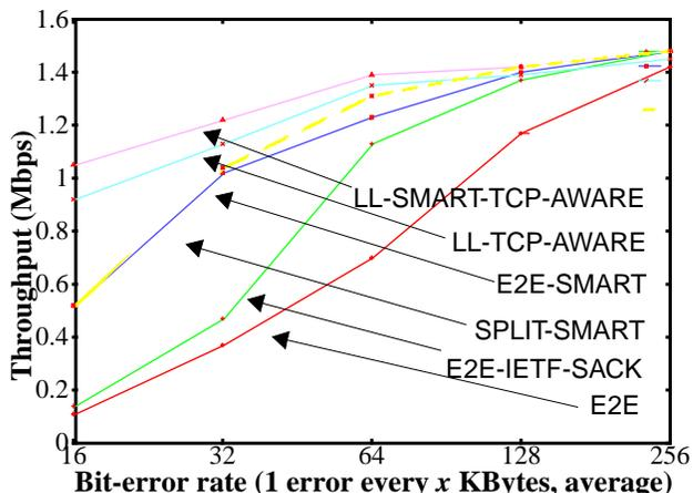
**Figure 20. Performance of six protocols (LAN case) across a range of bit-error rates, ranging from 1 error every 16 KB to 1 every 256 KB shown on a log-scale.** model are derived from a trace-based modeling and characterization of the WaveLAN network [21].
