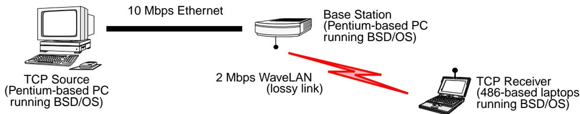
**Figure 10. Experimental topology.** There were an additional 16 Internet hops between the source and base station during the WAN experiments.
