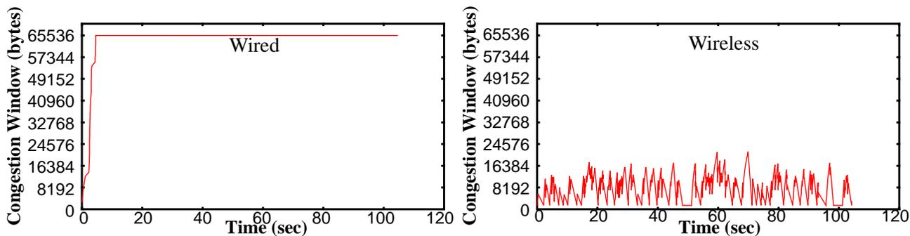
**Figure 19. Congestion window sizes as a function of time for the wired and wireless parts of the split TCP connection. The wired sender never sees any losses and maintains a 64 KB congestion window. However, the wireless TCP connection’s congestion window fluctuates rapidly.**
