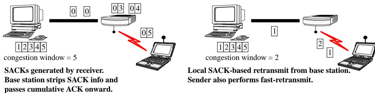
Figure 6. Link-Layer with SMART-based selective acknowledgments
