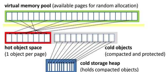
**Figure 1.** Archipelago’s software architecture. Archipelago randomly allocates heap objects in virtual address space (Section 3.1). It tracks the hot objects, which are stored one per page (Section 3.2). Cold objects are compacted and placed in cold storage, and the physical memory associated with their page frames is relinquished (Section 3.3).
