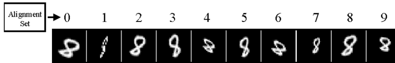
Fig. 6. A set of latent image estimates for an observed “8” image. The eight is aligned with each model in turn. Notice that alignment to the “1” model produces a latent image that is a plausible “1.” Rejecting this model will depend upon penalizing the highly unlikely transformation that would be paired with such a latent image to produce the observed image.
