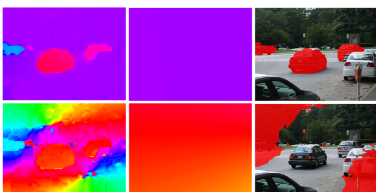
Fig. 8: RANSAC vs no RANSAC. Top row: robust initialization with RANSAC. Bottom row: using Bruss and Horn’s method directly on the entire image. Left to right: flow angles of observed translational flow, angle field M of static environment and segmentation.
