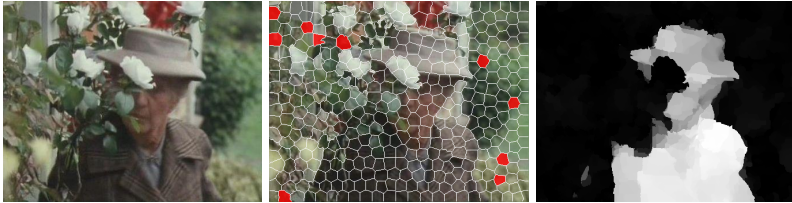
Fig. 6: RANSAC procedure. The result of our RANSAC procedure is to find image patches of the static environment. Notice that none of the patches are on the person moving in the foreground. Also notice that we force the algorithm to pick patches in three of the four image corners (a “corner” is 4% of the image). The right figure shows the negative log likelihood of the static environment.
