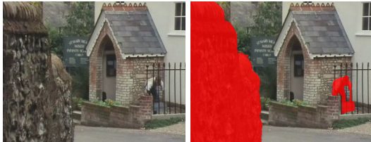
Fig. 7: Bad ground truth. Some BMS-26 videos contain significant ground truth errors, such as this segmentation of the foreground wall, which is clearly not a moving object.
