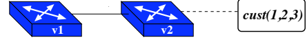
Fig. 3. Example in which the solution of the MC depends on initial state. Cube-shaped routers indicate cache-routers, while rectangles with rounded edges denote custodians, that permanently store the indicated files. Solid lines indicate an edge in E and dotted lines a cache-custodian association.
