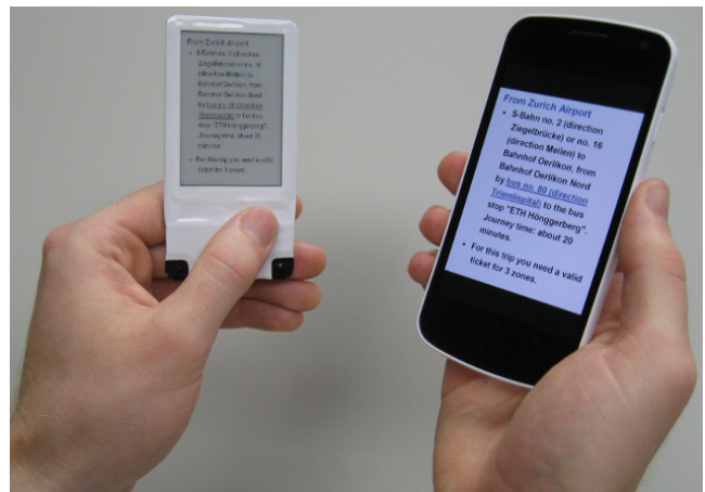
Figure 1. Display tag use scenario: companion display for mobile phone. The working prototype NFC display tag on the left shows travel directions captured from the screen of the phone on the right. All power and data to update the display is provided wirelessly by the phone's NFC reader.
