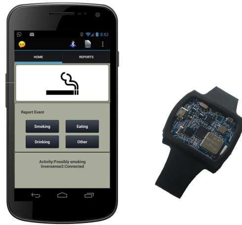
Figure 10: Smoking monitor mobile app and an IMU-equipped wristband.
