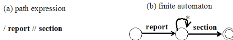
Figure 2: A path expression and its corresponding finite automaton
