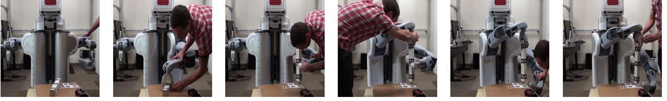
Fig. 2. A kinesthetic demonstration of the table assembly task.
