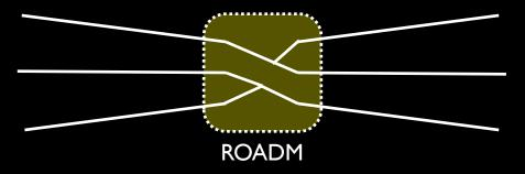
At each node, can only switch signals optically within sets of c incident fibers.
