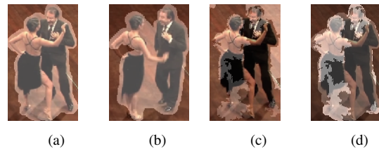
Figure 2: Similarity metric. (a) and (b) Pair of bounding boxes containing the foreground mask (colored light grey). (c) Confidence mask computed using NRDC (colored light grey). (d) Foreground mask and confidence mask overlapped. Only the pixels contained in both masks (colored in the brightest grey) are used for the for computing the similarity.
