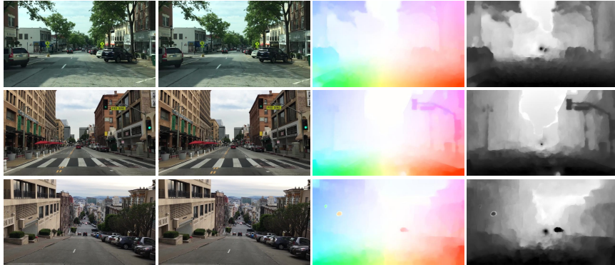
Fig. 2: Samples of image pairs and computed translational optical flow that we use to recover the relative depth. From left to right: first images, second images, translational optical flow between input two images, and relative depth of the first images.
