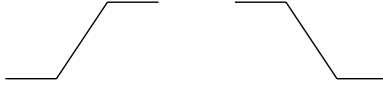
Figure 7: These two sections of the hexagonal grid, laid end to end, can be used to approximate any line segment which forms an angle \theta \in [0, \pi/6] with the x -axis.
