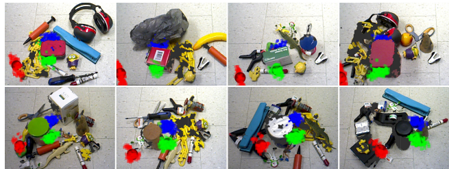
Fig. 7. Examples of grasping in a cluttered scenario. The red, green, and blue spheres represent the grasp points of the hand frame, thumb tip, and index finger tip of the left robot hand. The grasp points are the weighted mean of the colored dots that each represents a possible grasp position based on one training example. The top row is trained on grasping cuboid objects and the bottom row is trained on grasping cylindrical objects. Notice that our approach is able to identify the only cuboid or cylinder in the scene and generate grasp points similar to the training examples.
