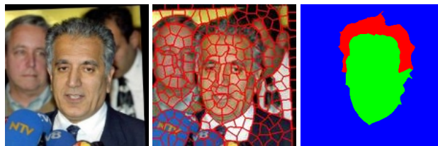
Figure 1. The left image shows a “funneled” or aligned LFW image. The center image shows the superpixel version of the image which is used as a basis for the labeling. The right image shows the ground truth labeling. Red represents hair, green represents skin, and the blue represents background.
