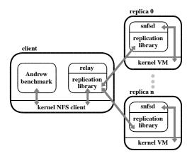
Figure 2: Replicated File System Architecture.
